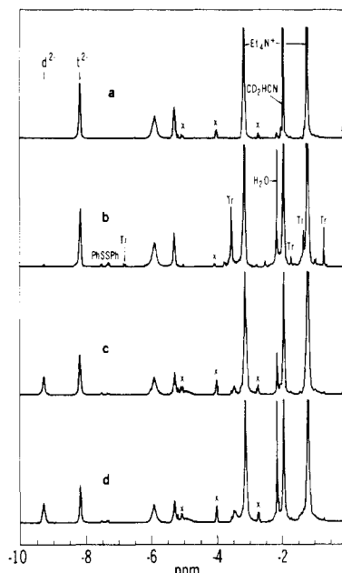
Figure 5. 1 H NMR spectra of CD 3 CN solutions of solids obtained upon addition of rhodanese to reaction mixtures of various compositions. Reagent concentrations (included as Table III in the supplementary material) and workup are similar to those given in the text and Table I. Relative concentrations of [\text{Fe}_2\text{S}_2(\text{SPh})_4]^{2-} ( d^{2-} ) and [\text{Fe}_4\text{S}_4(\text{SPh})_4]^{2-} ( t^{2-} ) were calculated from area ratios of the m -H resonances of d^{2-} (−9.3 ppm) and t^{2-} (−8.2 ppm). For each spectrum the form in which the iron was supplied, the ratio PhSH/Fe, the concentration of \text{Et}_4\text{NBr} (supplied at the outset), the overall yield by weight (calculated as the percentage of the iron supplied), and the mole ratio d^{2-}/t^{2-} are as follows (a) ferric ammonium citrate, 4/1 PhSH/Fe, no \text{Et}_4\text{NBr} , overall yield 60.2%, d^{2-}/t^{2-} = 0 ; (b) ferric ammonium citrate, 9/1 PhSH/Fe, 0.1 M \text{Et}_4\text{NBr} , overall yield 74.7%, d^{2-}/t^{2-} = 0.07 ; (c) ferrous ammonium sulfate, 12/1 RSH/Fe, 0.1 M \text{Et}_4\text{NBr} , overall yield 87.3%, d^{2-}/t^{2-} = 0.71 ; (d) ferric chloride premixed in \text{CH}_3\text{CN} with PhSH, 12/1 RSH/Fe, 0.1 M \text{Et}_4\text{NBr} , overall yield 86.7%, d^{2-}/t^{2-} = 0.66 . No other resonances were obtained in any of the spectra from +40 to −40 ppm. All spectra exhibit an area ratio m -H/cation \text{CH}_2 = 2.0 \pm 0.2 . Peaks marked with X denote solvent impurity, and Tr denotes residual Triton.
